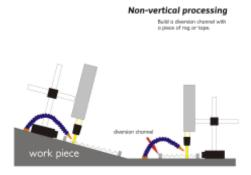
Vertical processing on big work piece. Adsorb the base directly on the work piece, and build a diversion channel under the work head to drain coolant outside.
