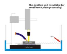
Choose desktop unit to fix the work-piece. It could process small work piece. Put the desktop unit into the tank to avoid the coolant losing.
