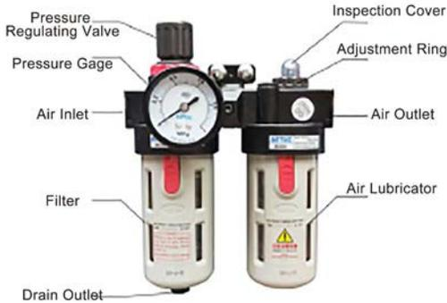
1. When adjusting the pressure, please pull up the pressure adjustment knob and then turn it. Press the rotary knob to position. Turn clockwise to increase the outlet pressure and counterclockwise to lower the outlet pressure.
